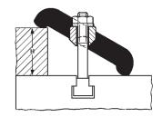
Holding capacity **[18000 lbf] 80kN** Clamping height 75 [3.00] max.
