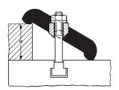
Holding capacity **[14000 lbf] 62.5kN** Clamping height [2.25] 57mm max.
